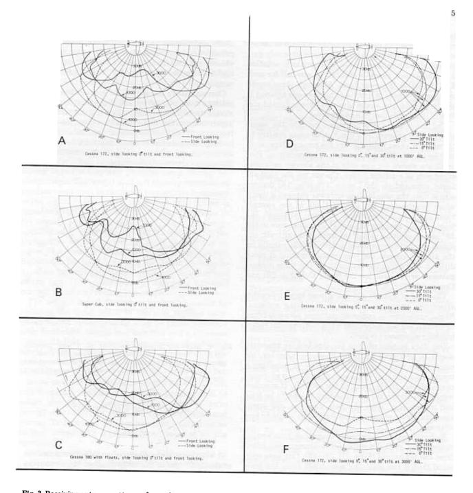
Fig. 3. Receiving antenna patterns of a yagi array system (164 MHz). Readings were not obtained within the sector 20° either side of the nose and tail of the aircraft. Aircraft were flown at altitudes of about 300, 600, and 900 m AGL.
