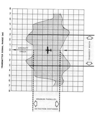
Fig. 5. An example of a signal reception pattern of a Cessna 172 with side-looking, 15° tilt yagi antennas flying at 300 m AGL. The shaded portion represents the area in which the transmitter signal can be reliably detected. In this example the minimum parallel detection distance was 8.0 km. The transect width was established at 9.6 km.
