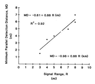
Fig. 6. Relation between minimum parallel detection range and signal range.
