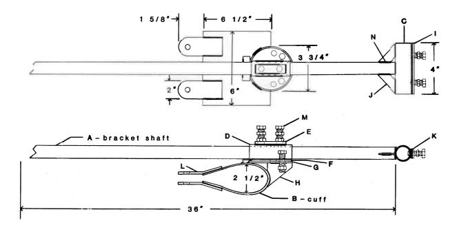
Fig. A-1. Schematic diagram of airplane wing strut yagi antenna mount. Measurements are provided in English units. Inside of cuff lined with padding to avoid scratching strut surface. All nuts and bolts should be certified for use on aircraft. These are available at any airport with repair facilities. Use lock nuts on cuff.
