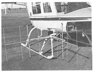
Fig. 2. Side- and forward-looking yagi antenna system designed for use on a helicopter (Bell 206B Jet Ranger). Rear quarter view (top), front quarter view (bottom).
