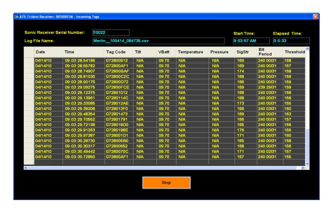
Another function accessed by the USB connection. This displays the data as it is being picked up by the Trident Receiver in blocks of fifteen seconds. So every fifteen seconds new tags will be sent out to the screen.
