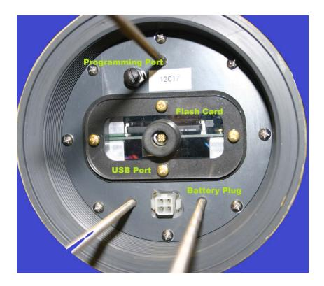
Notes: The programming port can be used to update the software that is on the supervisory board. The clear cover over the flash card port can be left off if quicker access during deployment is desired.
