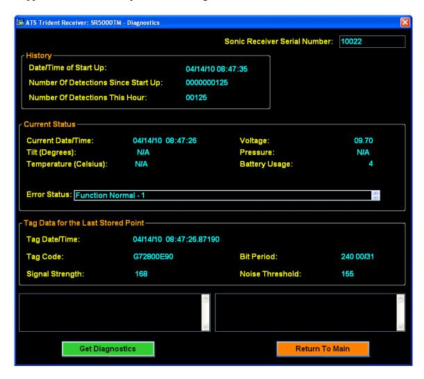
This function provides a snapshot of what the current status of the receiver is. A new log file is opened along with this window that saves a copy of the data shown on the screen. These log files are kept in the 'C:\Program Files\Advanced Telemetry Systems, Inc\ATS Trident Receiver SR5000TM\Log' folder.
