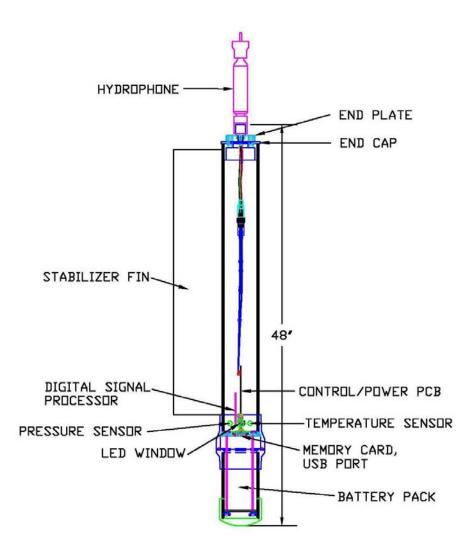
The hydrophone receives the high frequency mechanical vibrations sent through the water by the JSATS transmitter (in the fish) and converts them to weak electrical voltages. These weak voltages are amplified and filtered by the preamplifier of the Control/Power board (to reduce noise) and then sent to the DSP board for processing.
