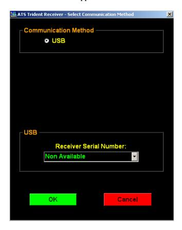
The USB Communication mode allows for real-time data viewing while the housing is open. Enter the serial number of the receiver and click OK.
