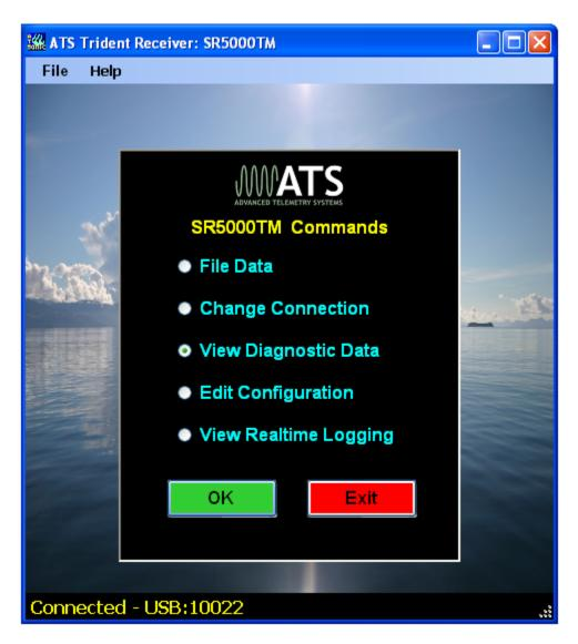
The USB connection allows you to update the configuration - "Edit Configuration", view the tags as they are being decoded - "View Realtime Logging" and view runtime information - "View Diagnostic Data".
