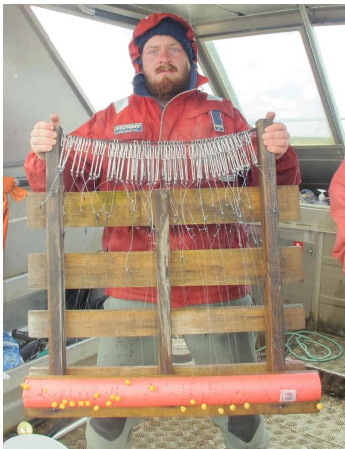
Figure 9. The purpose built rack used to store the snoods for the long line
