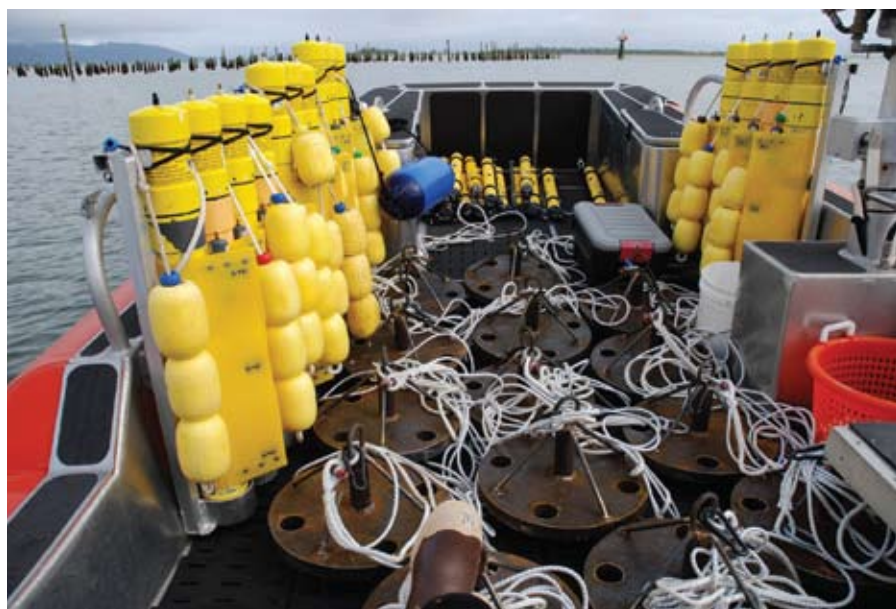
JSATS receivers and related mooring equipment loaded on a research vessel in the Columbia River estuary.
