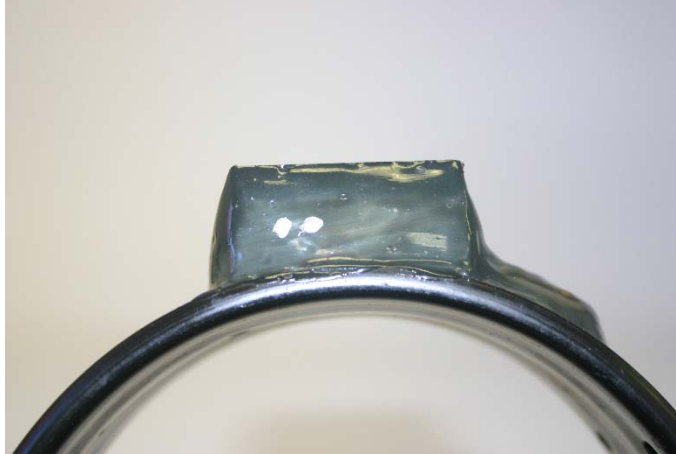
Figure 2. White dots indicating magnet placement on the potted electronics assembly.
