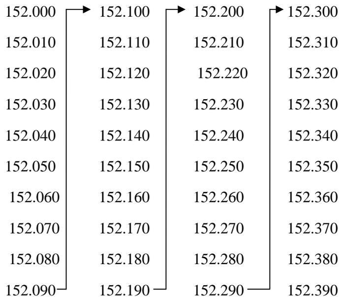
Figure 1. CONVENTIONAL TELEMETRY FREQUENCY ASSIGNMENTS.
