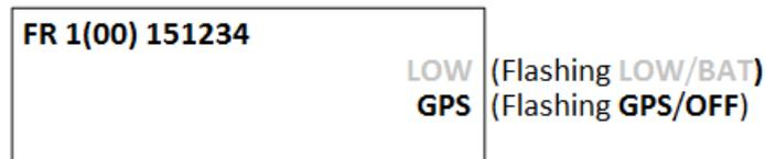
The GPS is normally OFF for the Manual Mode. If the GPS has been turned on previously from the GPS Screen, or an Aerial Scan, the GPS will remain on when entering the Manual Mode.
