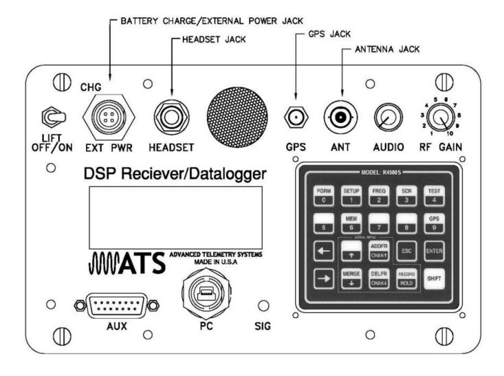
Most input and control of the receiver is done through the keypad. The keypad is shown below:
