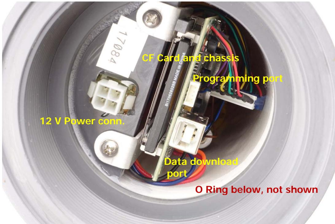
Notes: The programming port can be used to update the firmware that is used in the Control circuit.
