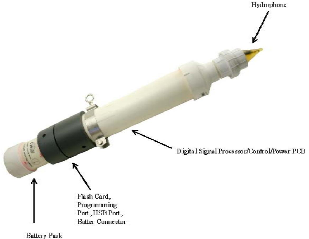
The hydrophone receives the high frequency mechanical vibrations sent through the water by the JSATS transmitter (in the fish) and converts them to weak electrical voltages. These weak voltages are amplified and filtered by the preamplifier of the Control circuit (to reduce noise) and then sent to the DSP circuit for processing.
