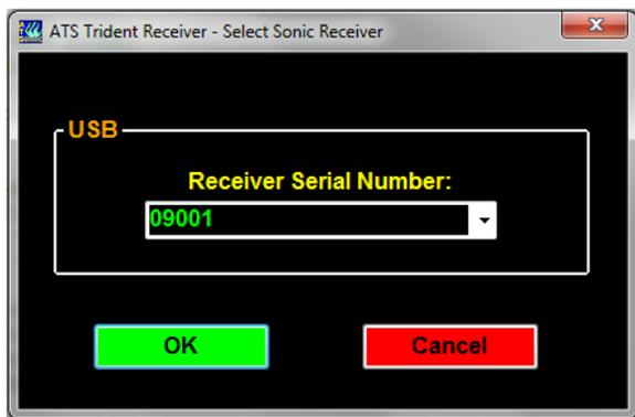
The USB Communication mode allows for real-time data viewing when the receiver housing is open. Enter the serial number of the receiver, which can be found on the placard affixed to the receiver's housing, and click OK.
